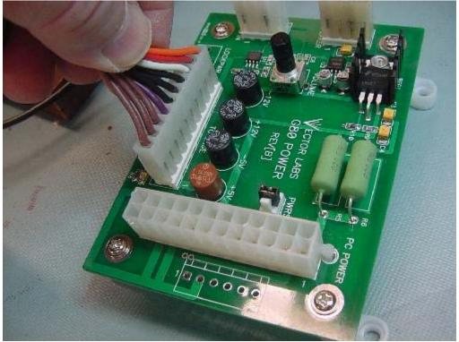
Now plug in the 20 or 24pin connector from the ATX supply as shown below.
