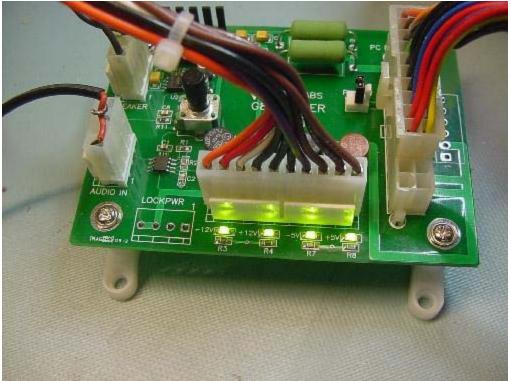
The 4 LED's should be lit indicating power available on the +5v - 5v + 12v & -12v outputs. Coin up the game and adjust the volume level control on the PCB.
