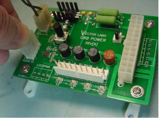
Next unplug the dc output connector from the old supply and plug into the new board as shown below.
