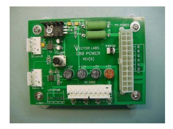
The Vector Labs G80 power supply replacement board enables the use of standard ATX switching power supply to generate the G80 card cage power and also has a bult in audio amplifier. The kit contains the PCB and 4 white mounting feet w/screws.
