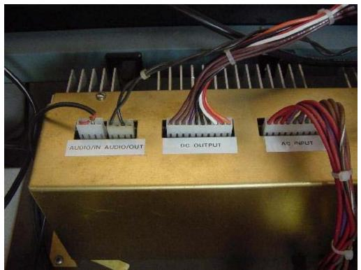
The typical G80 power supply is shown above and has four connectors, AC input from the transformer, DC output to the card cage, audio input and audio output. First unplug the AC input connector and zip tie somehere where it will not short out on anything, as it will not be used anymore. Next unplug the audio input and output connector and plug into the new board as shown below.
