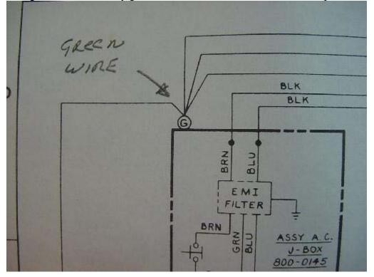
The green wire is a safety ground and will need to be attached to the point indicated below.
