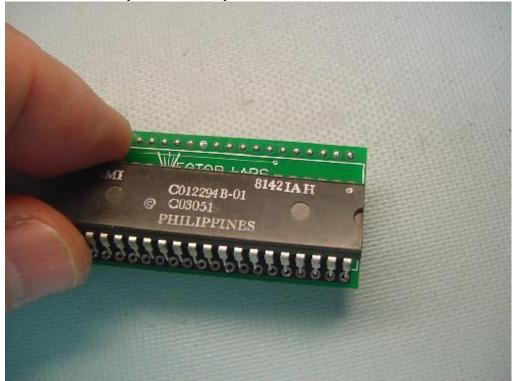
Now re-install the Pokey PWA back into socket C/D2 as shown below.
