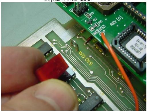
Now insert the Vector PWA into sockets N/P3 R3 as shown below.
