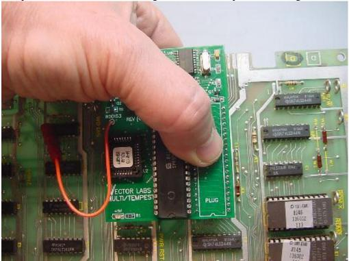
Now connect the orange wire with terminal onto the (Watch dog disable WDDIS) test point as shown below.
