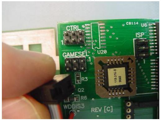
Now take the remaining 6 pin ribbon cable and connect to the connector labeled (CTRL) as shown below.
