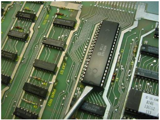
Insert the 6502 processor into the multigame main PWA board as shown below.
