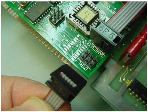
Route the cable around the edge of the Tempest PWB as shown below.
