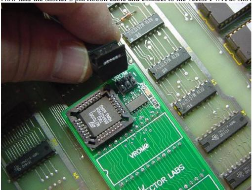
Plug the other end of the cable into the (GAMESEL) connector on the main PWA as shown below.
