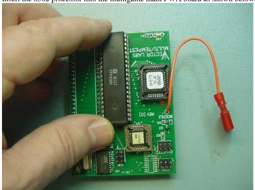
Install the multigame board into the Tempest main board 6502 socket as shown below. When pushing the board into the socket be sure to place your hand so it supports the Tempest PWB as well as the multigame board and squeeze them together.
