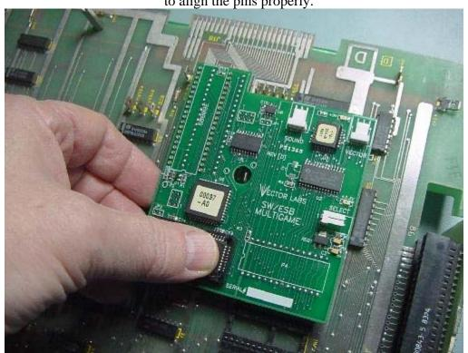
Reinstall 68B09E processor into socket on top of main kit board making sure that the "notch" is towards you as shown below.
