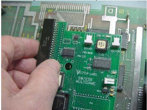
Install both 3 pin cables as shown below, The violet, grey, white into the connector labeled "SOUND" and the yellow, green, blue into the connector labeled "VECTOR"
