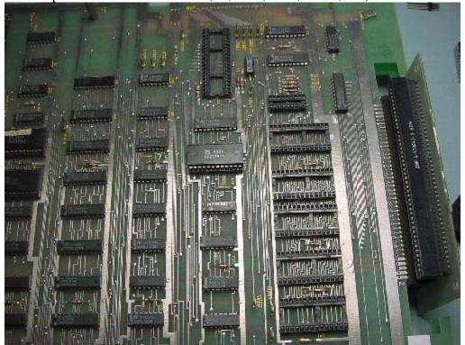
Install kit main board into processor socket 2C & Eprom sockedt 1F being careful to align the pins properly.
