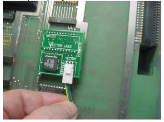
Flip boardset back over and set aside. Remove 68B09E processor from sound board socket location (3K) and Eproms (1J/K & 1H as shown below.
