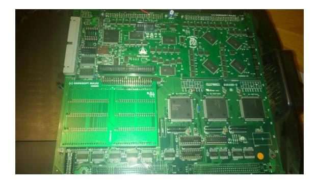
Now you can proceed to insert the tiny PCB that joins these two PCBs together. Make sure that the AU sign is facing upwards as it's shown in the picture below:
