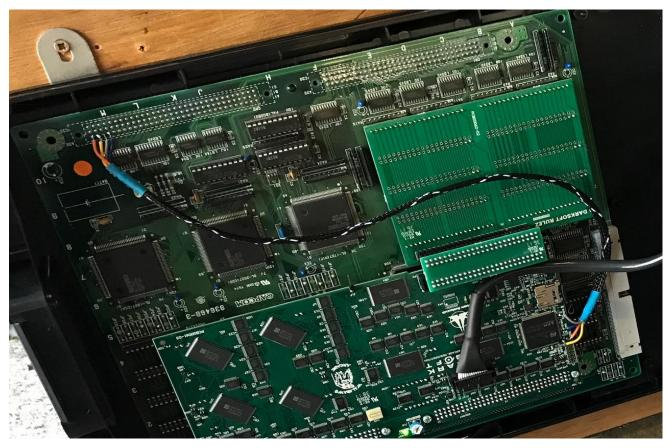
4 wires connected to CN2
