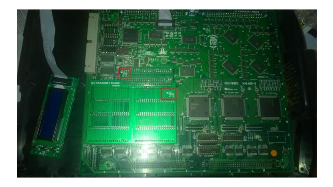
Your kit also includes an LCD screen module with 3 buttons to choose which game to load. The buttons and the cable are connected to the bigger PCB's 14-pin socket and you can take that cable outside the B Board case through the register opening in one of the sides. You will be able to change games with the lid closed.
