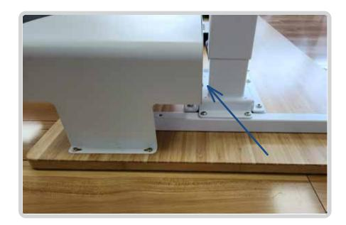
Once in position, use all 4 screws to attach the drawer to the desktop. The self-tapping screws are typically sharp enough to allow you to use a hand screwdriver to screw firmly into the desktop with a reasonable level of force. If you find this difficult, you may benefit from using a power drill.
