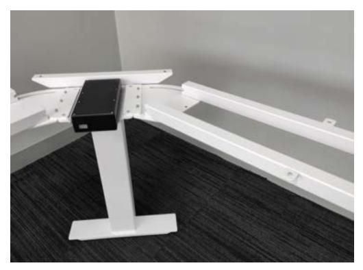
Accessing the frame from underneath, connect the spreader bar to the pivot plate using 2 x M8x10mm screws. Do not tighten at this point; the spreader bar should be able to pivot within the pivot plate slot.
