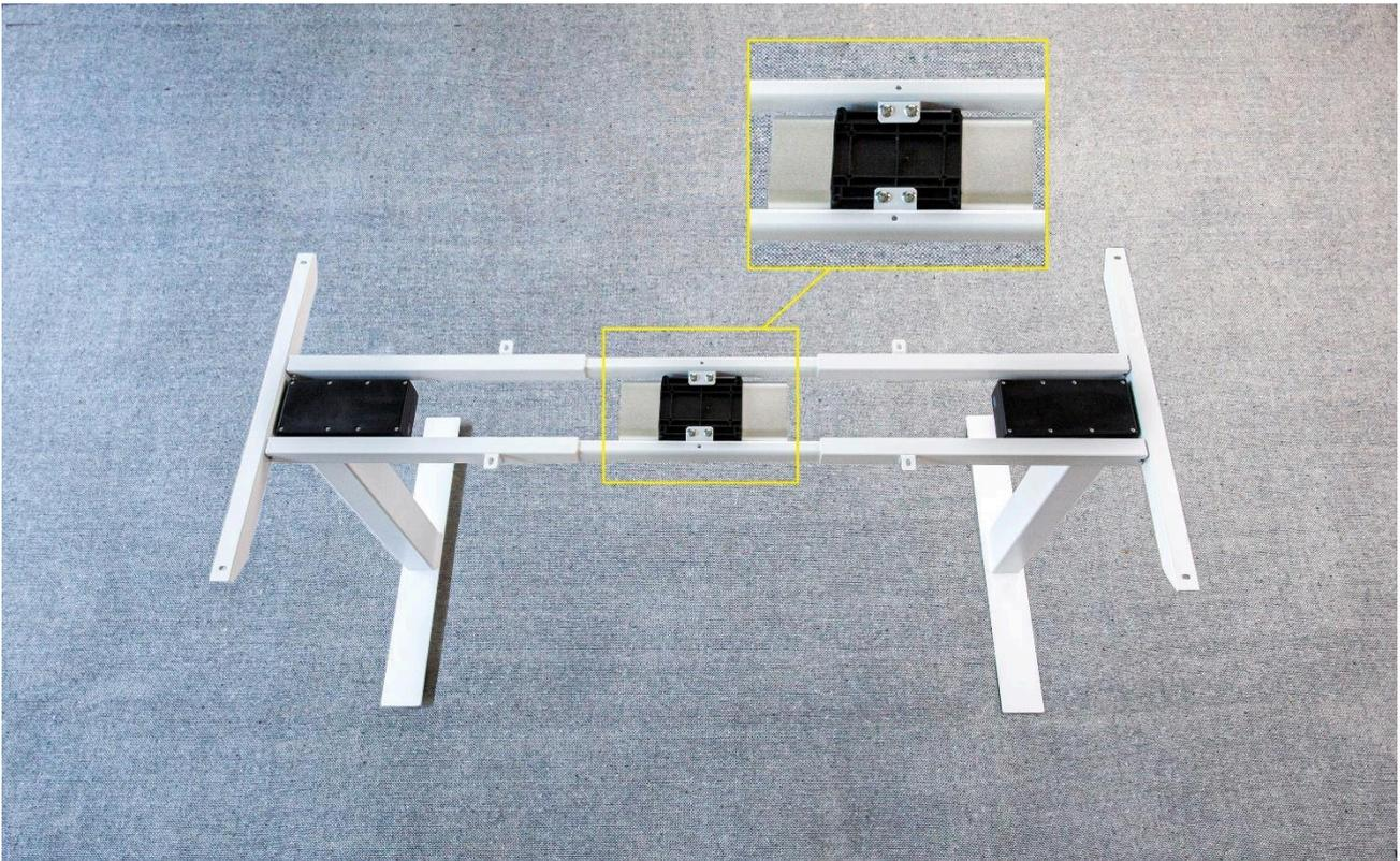
Flip the desk frame onto its feet. Install the control box (#5) as shown. Using a Philips head screwdriver (not the Allen key), install the four 'M6 x 10mm' screws. Tighten the screws until they are full seated on the steel bracket. DO NOT overtighten these screws or use excessive force once they are seated.
