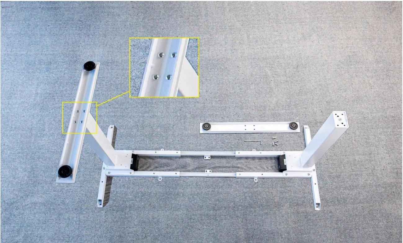
Install the feet (#2), keeping the black pads facing upwards as shown. Screw in four 'M8 x 20mm' bolts for the first foot using the Allen key (#8) and tighten firmly. Repeat on the other side.
