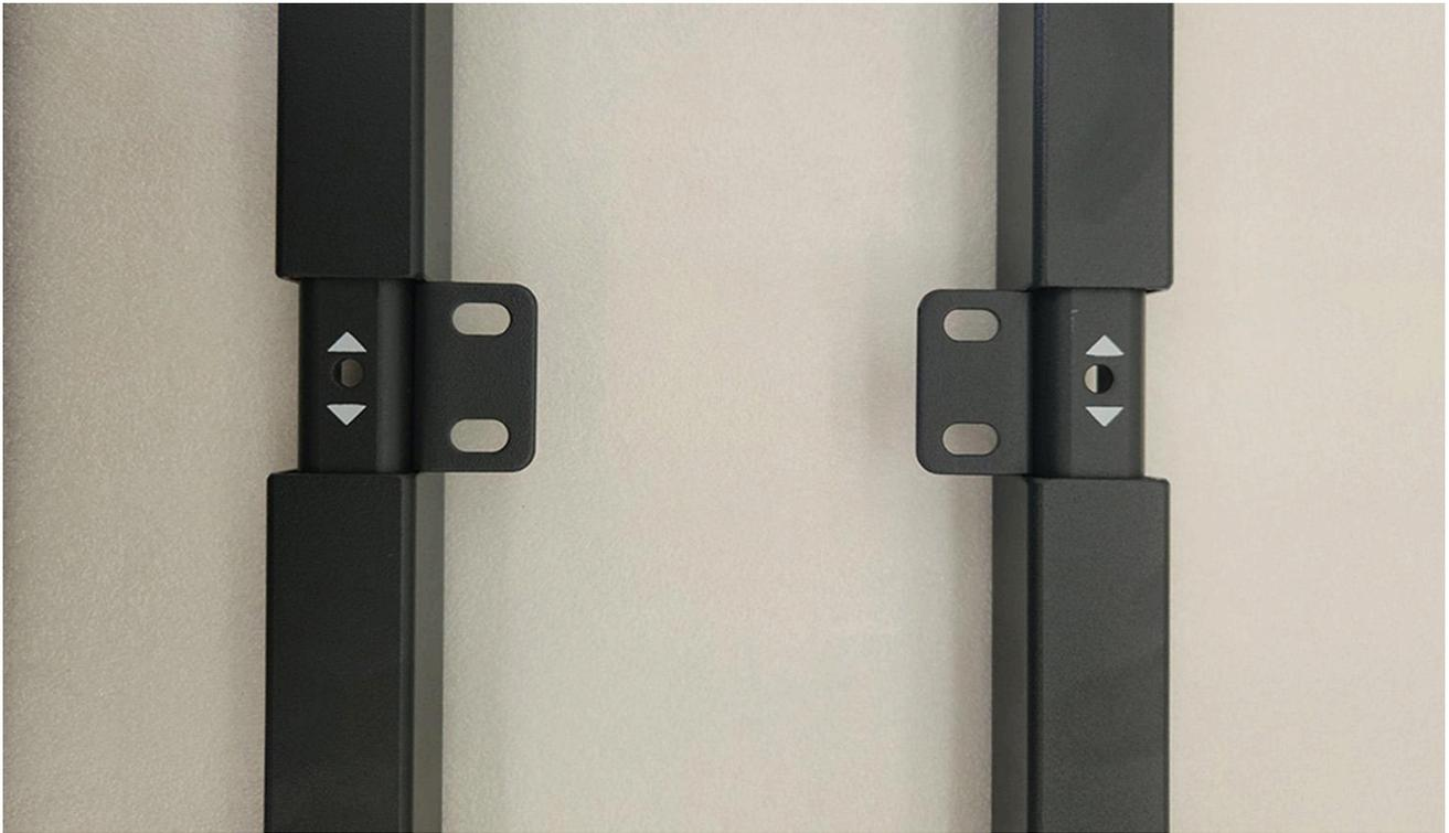
150cm desktops require the tubes to be extended out to 130cm. To do this undo the grub screws just until the point where you are able to slide the adjustable part of the tube. Please align the end of the tube with the 1.3 marking. You will need to repeat this step for both sides of each adjustable rail.
