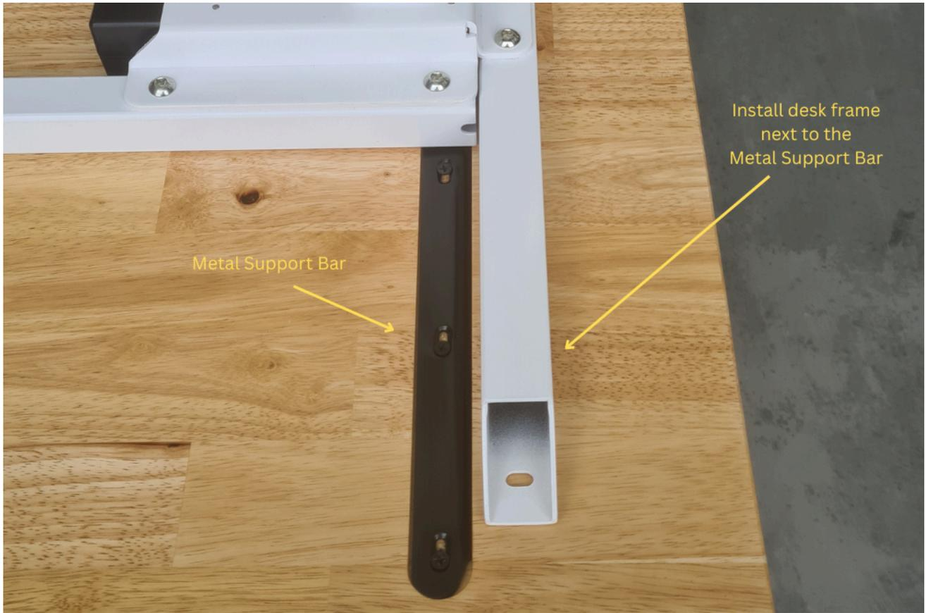
Using a screwdriver and the provided 16mm long self-tapping screws, affix the frame in 8 (eight) places. Start by screwing in one of the wings (#3) as indicated below. Re-measure, adjust if necessary and then screw a second screw in the diagonally opposite corner wing to ensure the frame is locked in position. All other screws can then be screwed in, in any order thereafter.
