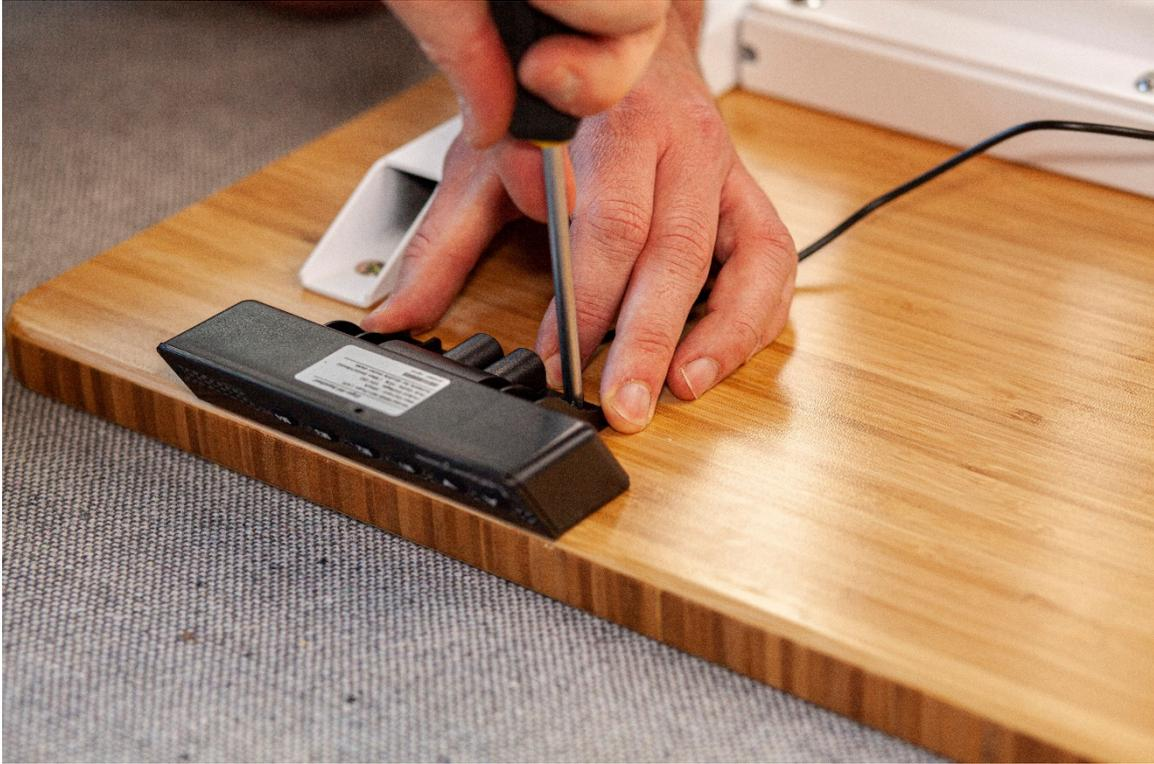
With the desk still upside down, simply align the top edge of the control panel (#10) with the edge of the desk. Using 2 (two) self-tapping screws and a Philips head screwdriver, screw the control panel to the timber.
