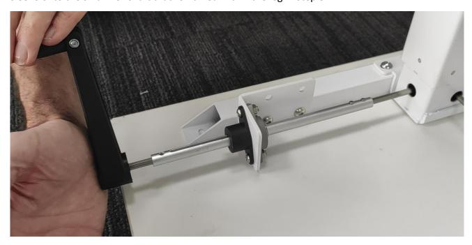
Tap the handle so that it positioned as shown below. The goal is to ensure the crank handle is situated <u>completely</u> under the desk when not in use, and can be pulled out when you require a desk height change.
