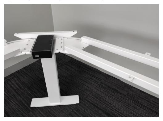
Accessing the frame from underneath, connect the spreader bar to the pivot plate using 2  $\times$  M8x10mm screws. Do not tighten at this point; the spreader bar should be able to pivot within the pivot plate slot.
