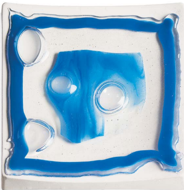
Figure 8: This plate (shown sitting on the mold) was formed with a single firing for both fusing and slumping. This shortcut caused edge distortion and bubbles.
