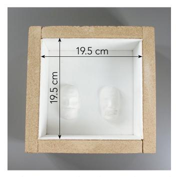
Mix the investment according to the previous directions and pour it quickly and evenly. Avoid pouring the mix directly onto the design elements or the side walls. Vibrate the work surface to assure that the investment levels out.
