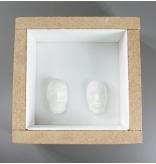
Hydrate the plaster/silica design elements by soaking them in water until the bubbles quit rising (5-10 minutes). This helps to keep the plaster/silica bed from sucking in around the design elements due to differences in humidity. Arrange design elements on the interior base of the box. Check once again to make certain that your work surface is flat and level.
