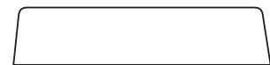
Figure 13: Fiber paper thickness too great. Dams not vertical—finished block won't sit vertically.
