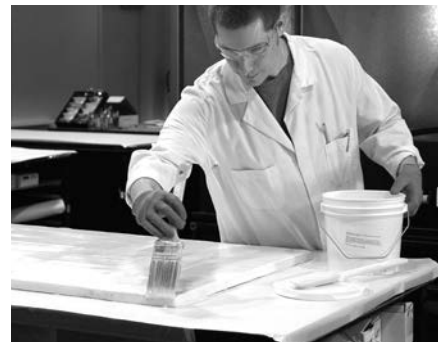
Figure 8: Brushing qf-180 onto the fiberboard shelf.
