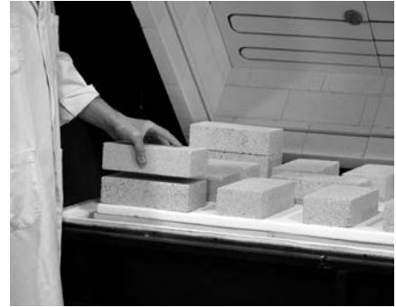
Figure 11: weighting the fiberboard shelf with bricks.
