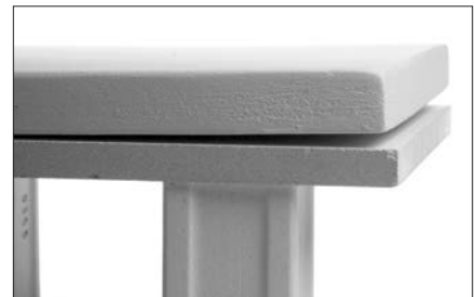
Figure 12: example of a bowed fiberboard shelf corner.
