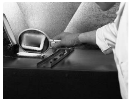
Figure 7: using a mirror to check for condensation.
