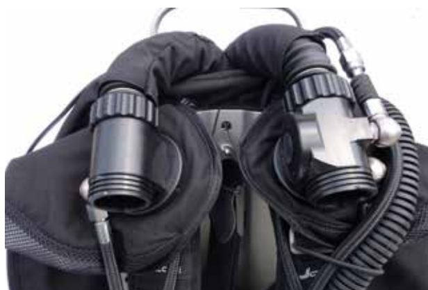
Connect the breathing hoses to the T-piece and ADV. It is not possible to connect these incorrectly because the two connection threads are different. The connection thread on the inhalation side (ADV) is clockwise, whilst the thread on the exhalation side (T-piece) is anti clockwise.
