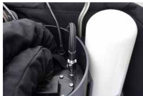
Now connect the oxygen low pressure hose. Only tighten until hand-tight!
