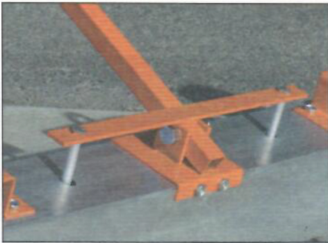
Tow bar attached to sweeper assembly.
