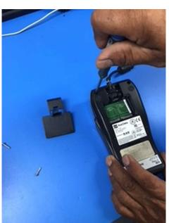
Remove the four corner screws.
