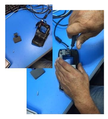
Remove the two screws of cord.
