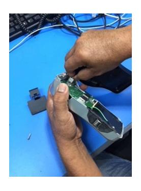
Unplug the white cable. Pull from the white part. Be careful not to strip the cables out.
