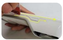
3. Use a slim card to slide through the side creases to unlock the bottom cover.
