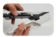
7. Perform the steps in reverse to close your device. Install the cover from thick section to thin section. Apply pressure to the top cover to more effectively and securely close the device. Be careful not to press on the camera as you press the cover in place.
