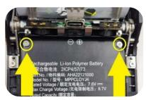
5. Remove the two screws holding the battery.
