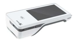
For periods of infrequent use or for storing the Clover Flex we recommend fully charging your device and powering off. You should repeat this every 6 - 9 months. These steps are important, because a fully charged primary battery will protect your device with tamper detection for about 1 year.
