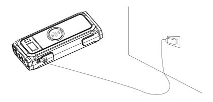
**2.** Insert one end of the cigarette lighter charger into the 12V auxiliary power outlet in your vehicle and insert the other end of the cigarette lighter charger into the device.
