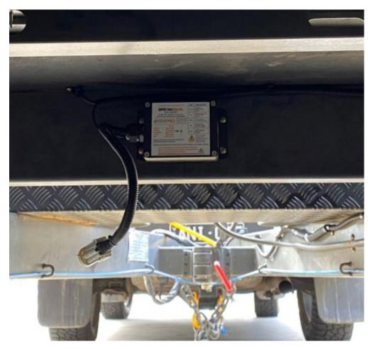
Ensure that the SwayControl is mounted in the correct, UP direction. The centre of the SwayControl (marked by the orange dot on the SwayControl label) must be positioned over the centre line of the caravan/trailer. The bottom edge of the SwayControl (as indicated by the orange line on the bottom of the SwayControl label) must be mounted parallel to the trailer beam axle.
