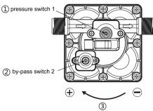
**CAUTION:** The pressure setting for full bypass must be at least 8psi higher than the shut-off pressure of the pump. If the switch and bypass is adjusted too closely, the bypass and switch shut-off can overlap and the pump will not shut off.
