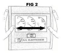
To fit the mounting screws, remove the front cover by gently pulling the side wings apart. (See FIG 2) When replacing the cover check the switch button is not jammed. Make sure the heads of the screws do not protrude over the edge of the base as this may prevent the front cover from fitting correctly.
