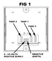
Cut a rectangular hole behind the gauge for the sender probe connector plugs to fit through. Feed the wiring loom up through to the water gauge and connect the plugs into the back of the gauge.
