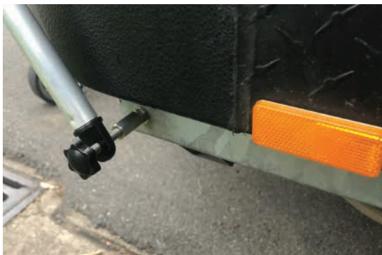
Pole 4a and bolts mounting
