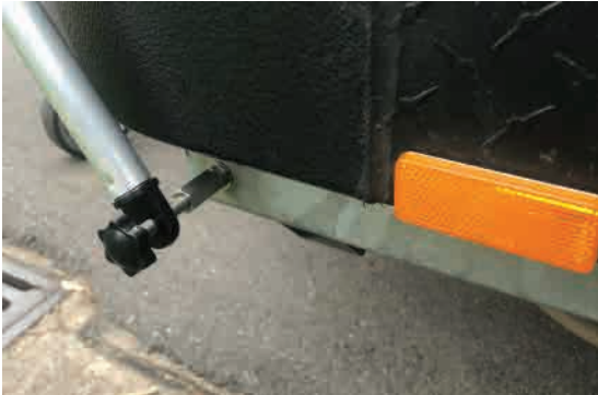
Pole 4a and bolts mounting
