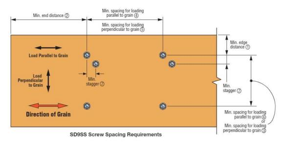
SD Connector SS Screw Spacing Requirements
