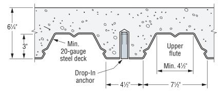
**Lightweight Concrete over Steel Deck**
