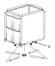
4. Note the sleeves on the fourth side are secured by hook & loop material. Open the sleeves and insert two Short Tubes (A) and connect them with a 3-Way Side Connector (E) in middle. Connect the tubes to the two 4-Way Corner Connectors (F) and close the sleeves.
