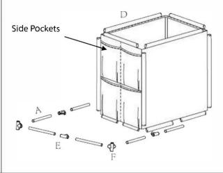
3. Attach the tubes from Step 1 to the 3-Way Side Connectors (E) from Step 2.
