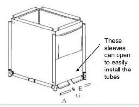
5. Insert the Long Tubes (C) through the corner sleeves of the Mesh Bag and into the 4-Way Corner Connectors (F).
