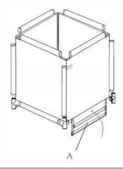
3. Insert Tubes (A) through the corner sleeves of Mesh Bag (B) and into the 4-Way Connectors.
