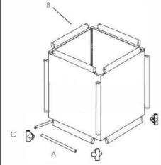
2. Notice one of the sleeves is secured by hook & loop material. Open the sleeve to install the fourth tube.
