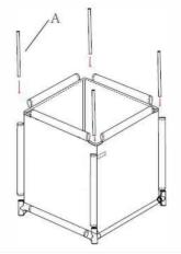
4. Insert Tubes (A) through the upper sleeves of Mesh Bag (B).
