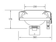
NOTE : This unit should be connected to an uninterrupted source of potable water, no less than 15mm (1/2"), with a minimum flowing pressure of 130KPa and a maximum static pressure of 860 KPa.
