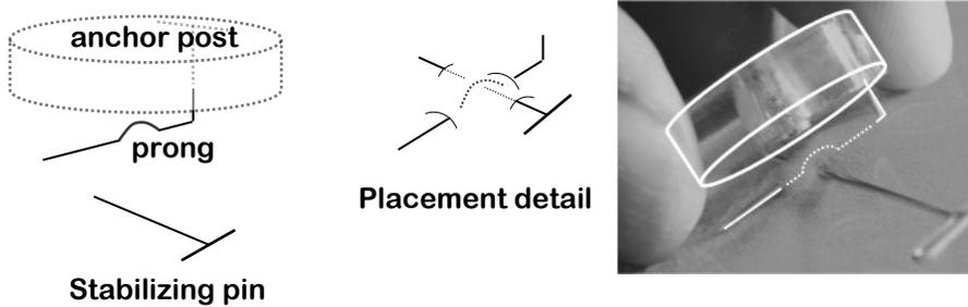
Hold anchor post with the prong the fabric (Figure 1). Lower post, piercing fabric with prong.
