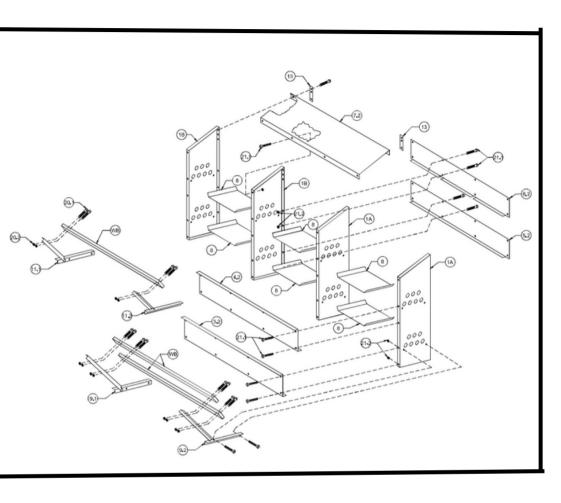
Step 2:Attach the Front and **Back Panels using the smaller** screws and nuts. (PT # 21.1 and 21.2). Panels are as follows: Front bottom panel (PT # 3.3) Note: This panel has one lip, no notch. Back Bottom panel (PT # 5.3) Note: This panel has one lip, no notch. Front Top panel (PT # 4.3) Note: This panel has two lips and three notches. Back Top panel (PT # 6.3) Note: This panel has one lip and three notches. Hand tighten.
