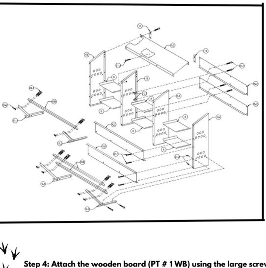
**Back Panels using the smaller** screws and nuts. (PT # 21.1 and 21.2). Panels are as follows: Front bottom panel (PT # 3.2) Note: This panel has one lip, no 🗸 notch. Back Bottom panel (PT # 5.2) Note: This panel has one lip, no notch. Front Top panel (PT # 4.2) Note: This panel has two lips and two notches. Back Top panel (PT # 6.2) Note: This panel has one lip and two notches. Hand tighten.
