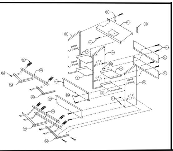
**Step 2:Attach the Front** and Back Panels using the smaller screws and nuts. (PT # 21.1 and 21.2). Panels are as follows: Front bottom panel (PT # 3.1) Note: This panel has one lip, no notch. Back Bottom panel (PT # 5.1) Note: This panel has one lip, no notch. Front Top panel (PT # 4.1) Note: This panel has two lips and one notch. Back Top panel (PT # 6.1) Note: This panel has one lip and one notch. Hand tighten.
