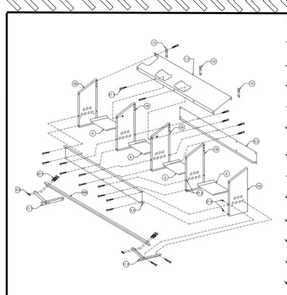
Step 4: Attach the wooden board (PT # 1 WB) using the large screws and nuts (PT # 20.1 and 20.2)
