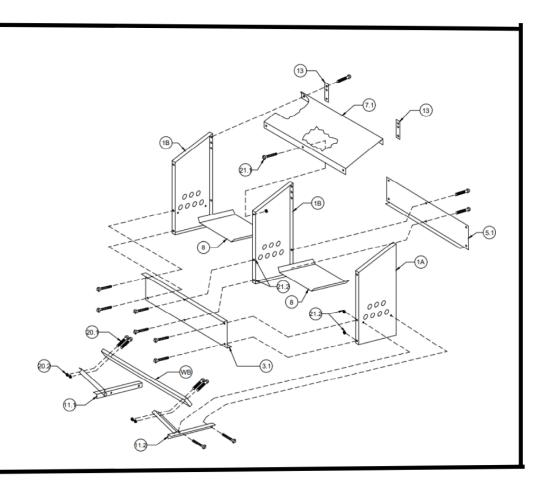
Step 2: Attach Front bottom panel (PT # 3.1) using the smaller screws and nuts (PT # 21.1 and 21.2). -- This panel has two lips with NO notches. Then attach the Back bottom panel (PT # 5.1) using the smaller screws and nuts (PT # 21.1 and 21.2). -- This panel has one lip with NO notches. Hand tighten.
