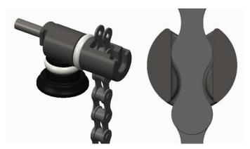
Wind the breaker screw in by hand until it contacts the chain rivet. You may need to adjust the chain position slightly to ensure the screw and rivet are aligned. You can now use your wrench to drive the breaker screw, pushing the rivet through the chain.
