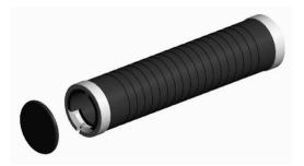
With the end caps removed you can now slide the grips back on your handlebars and secure in place. Now is also a good time to check that there are no sharp edges around the inside edge of your handlebars as these can damage the o-rings – use a file or a sharp knife to remove any burrs.
