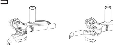
Squeeze your lever, watching for any air that bubbles into the bleed kit body. Release the lever, then squeeze again - repeat until no more air comes through.
