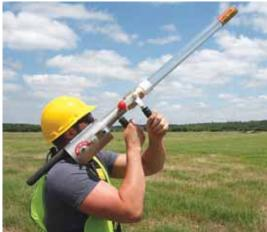
Shoulder Shot launcher uses compressed air to shoot a safety line as high as 250 ft.
