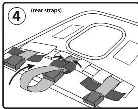
Finally, stow all mounting strap tails using velcro loops
