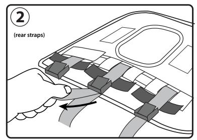
Regularly check for tightness, wear, and loose straps. Failure to do so may result in damage or injury.
