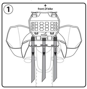
...return straps through holes and engage with cam buckles, do not tighten yet
