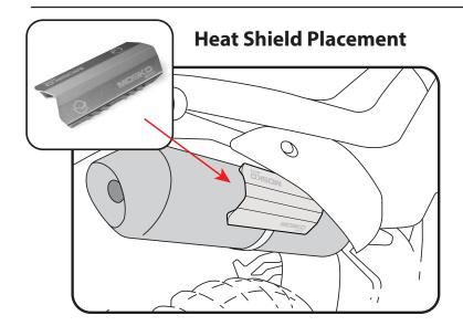
It is your responsibility to place the provided heat shield on your exhaust pipe using the hose clamp, in a location that protects the bag and your motorcycle's body panels from melting due to tail pipe heat. It is important to check after each use that your heat shield is located properly.
