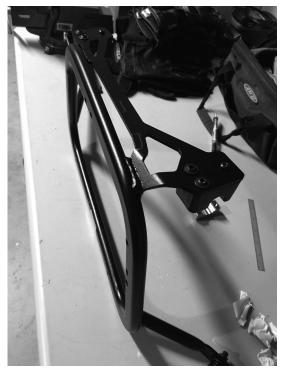
Pucks at the top side of the side carrier rack. As you can see the support bracket that has been welded to the rack has left little room for the pucks.
