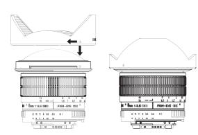
Align the attachment reference point on the hood with the hood reference point on the lens, push the hood onto the lens and turn the hood clockwise until it makes a clicking sound.
