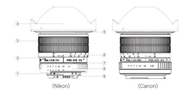
① Mount (camera locking area) ② Distance scale point 3 Focusing ring ⑤ Hood locking tube 6 Focus scaling ring Point ring ® Aperture adjustment ring ® CPU (electronic contact)
