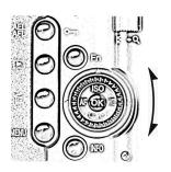
※ For some Olympus (MFT) and Panasonic (MFT) cameras, if you set the camera mode dial to A and set the brightness by turning the aperture adjustment ring on the lens, the camera automatically changes the shutter speed. Therefore you don't need to adjust the shutter speed as well, which is required in M mode.
