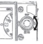
\*\* For some Sony E cameras, if you set the camera mode dial to A and set the brightness by turning the aperture adjustment ring on the lens, the camera automatically changes the shutter speed, so you don't have to adjust the shutter speed as well, which is required in M mode.
