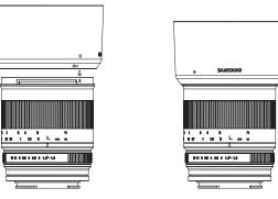
Align the attachment reference point on the hood with the reference point for a hood on the lens, push the hood onto the lens and turn the hood clockwise until it makes a clicking sound.
