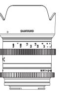
Align the attachment reference point on the hood with the hood reference point on the lens, push the hood onto the lens and turn the hood clockwise until it makes a clicking sound.
