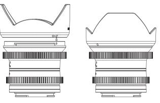
Align the attachment reference point on the hood with the hood reference point on the lens, push the hood onto the lens and turn the hood clockwise until it makes a clicking sound
