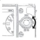
For some Sony E cameras, if you set the camera mode dial to A and set the brightness by turning the aperture ring on the lens, the camera automatically changes the shutter speed. Therefore you don't need to adjust the shutter speed as well, which is required in M mode.
