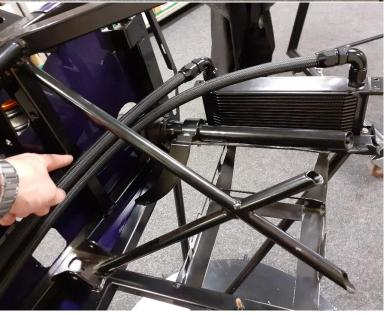
Securely mount the oil sandwich plate ensuring to apply a small amount of oil to the O-ring that sits on the engine oil housing. There is not a specific torque setting for the center adaptor bolt due to the O-ring seal on the plate but you must ensure this is tight. The use of a small amount of thread lock is advisable.
