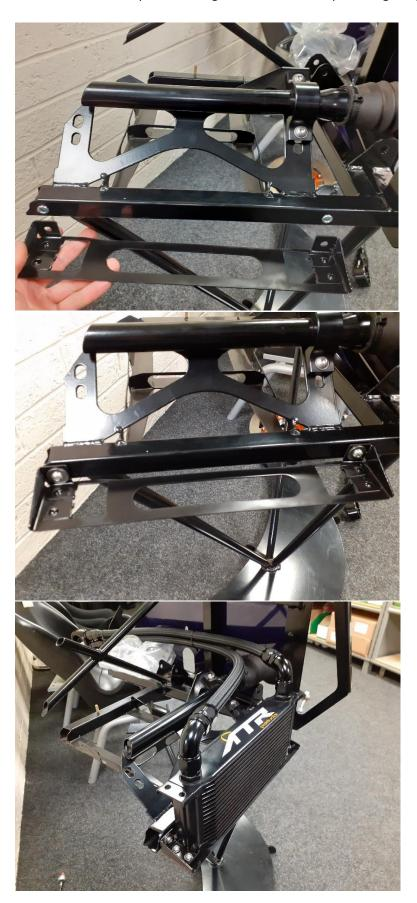
If your Zero chassis was produced before October 2019 you will need to fit the 'retrofit' oil cooler bracket to the lower front cross member of your Zero.
