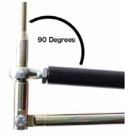
5. When this is correct, tighten the 4 gearbox bolts up and the rose joint locking nut up.
