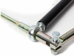
3. Fit one end of the spider to the gear box. Then mounting tube to gear box using longer bolt to the front, just fitting them hand tight at this stage.
