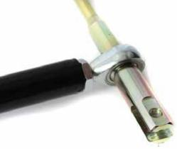
2. Fit bottom tube to fork end with bolt and washers - 1 each side and put the nut on hand tight.
